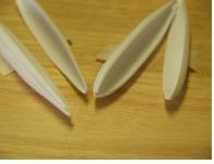
doubler shells ( Identified by the groove molded down the center.)
